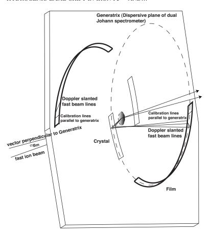
FIG. 2. SS1 spectrometer, showing the origin of Doppler-slanted lines.  $\alpha_{Bm}$  is the angle of the incident beam with respect to the crystal generatrix.
