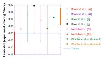
Comparison of theory and experiment for the 1s-2p Lamb shift. Results are paired with Lyman  $\alpha_1$  (1s-2p<sub>10</sub>) followed by Lyman  $\alpha_2$  (1s-2p<sub>10</sub>)
