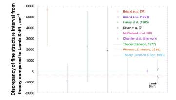
FIG. 9. (Color online) Plot of recent measurements of the hydrogenic fine-structure Lamb shifts for iron. References from Table VII: Briand *et al.* [34]; Silver *et al.* [9]; McClelland [33]; Briand *et al.* [35]; Hailey *et al.* [16]; theory (Johnson and Soff [24]). References given on right correspond to data appearing left to right in figure.
