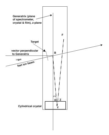
FIG. 3. SS1 spectrometer, side on, showing the x-ray path into and out of the crystal (assuming particlelike ray tracing).  $\alpha_{Bm}$  is the angle of the incident beam with respect to the crystal generatrix.  $\alpha_1$  is the angle of the x-ray path away from the generatrix, to the film location.
