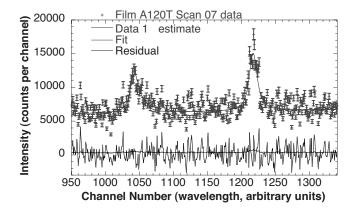
FIG. 7. An individual scan (number 7) of a particular Rowland circle (A1), emulsion (20), and densitization (T) using a PET diffracting crystal, in the region of the Balmer  $\gamma$  region of overlap between the first and fourth orders of diffraction: [Ba  $\gamma$   $2p_{1/2}$ - $5d_{3/2}$ ; Ba  $\gamma$   $2p_{3/2}$ - $5d_{5/2}$ ]. The residuals are clearly dominated by noise, indicating a consistent fit.
