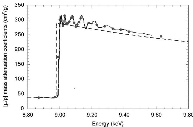
FIG. 10. Detailed XAFS measurement of the Cu  $K$  edge on an absolute scale, compared to theory (---, Chantler [6]). ●, this work (dot size represents  $10\sigma$ ). The relative measurements (—, [38]) are in excellent agreement with our results. Theory based upon the isolated atom approximation serves as a reference profile for XAFS contributions.
