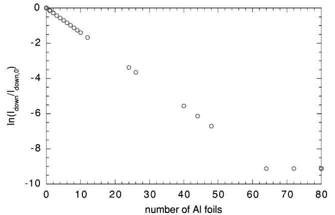
FIG. 5. Measurement of  $\ln(I_{down}/I_{down,0}) = -\mu t$  of aluminum as a function of the number of foils in the beam. The linearity of this plot confirms the linearity of the detector response. Linearity for large numbers of foils also confirms the absence of harmonic wavelengths in the monochromatized beam. The slope becomes zero when results are limited by calibration of detector noise and offsets.
