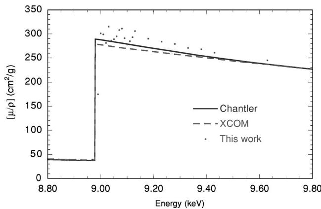
FIG. 9. X-ray anomalous fine structure (XAFS) measurement at the Cu  $K$  edge on an *absolute* scale, compared to DHF theory (solid line, Chantler [6]) and earlier theory (dashed line, Scofield [7]). The theories do not allow for solid-state effects, but XAFS assumes a baseline underlying the oscillations and [6] provides a more appropriate baseline in this regime.
