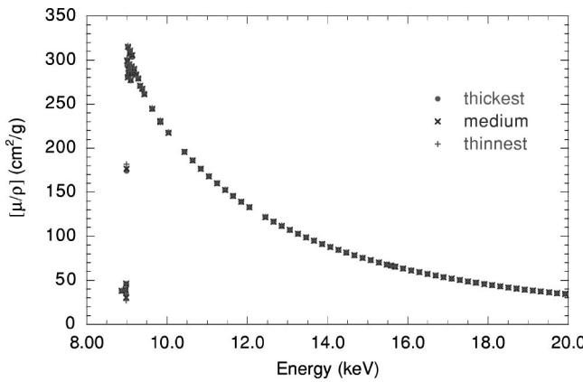
FIG. 7. Results of the measurements of the mass attenuation coefficient of copper. On the scale of this graph the measurements obtained with the three foils thicknesses overlap, showing precision of much better than 1%.
